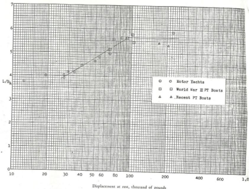
Fig. 16. Variation of Length/Beam Ratio with Displacement
