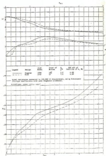
Fig. 14. Effects on Planing Boat Performance of Different Amounts of Twist in the Hull Bottom
