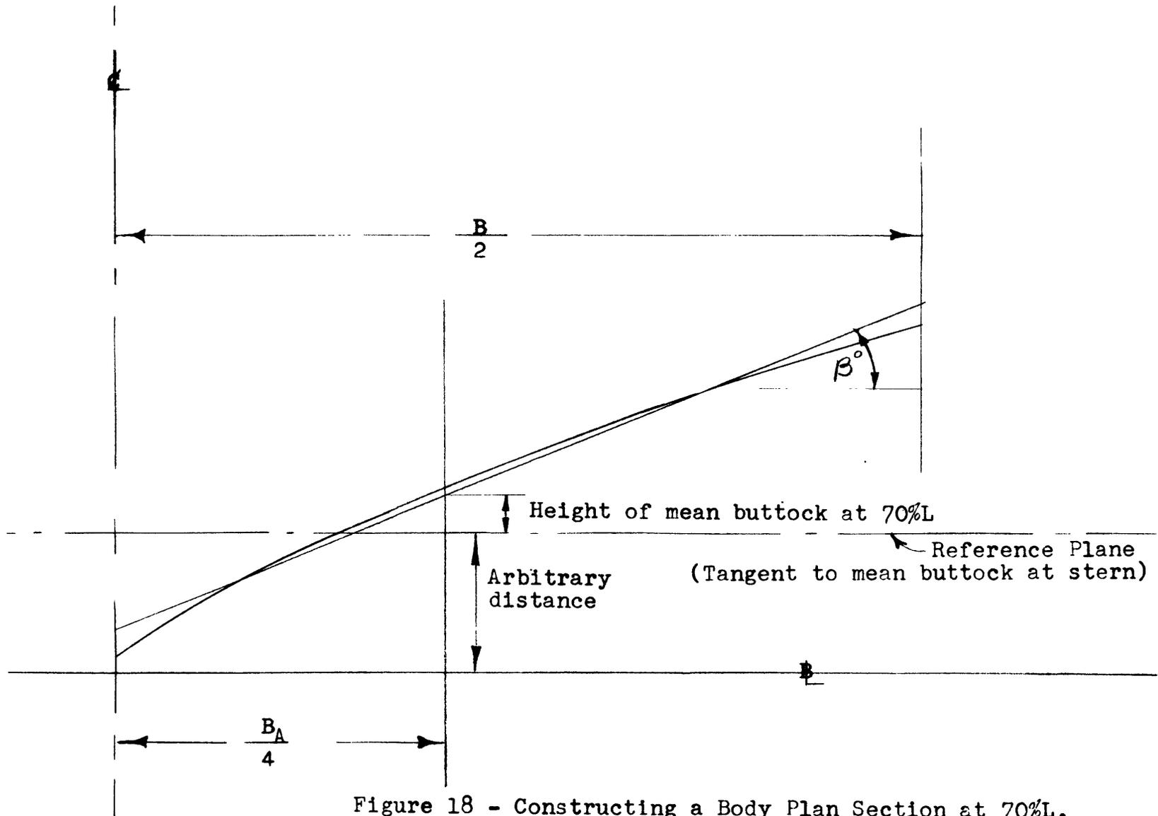
Figure 18 - Constructing a Body Plan Section at 70%L.
