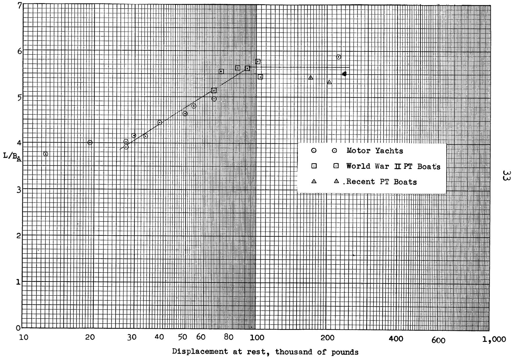
Figure 16 - Variation of Length / Beam Ratio with Displacement.
