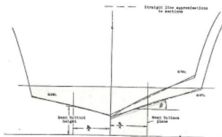
Fig. 1. Typical Planing Boat Body Plan with Straight Line Approximations to Sections
