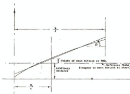
Fig. 18. Constructing a Body Plan Section at 70% L
