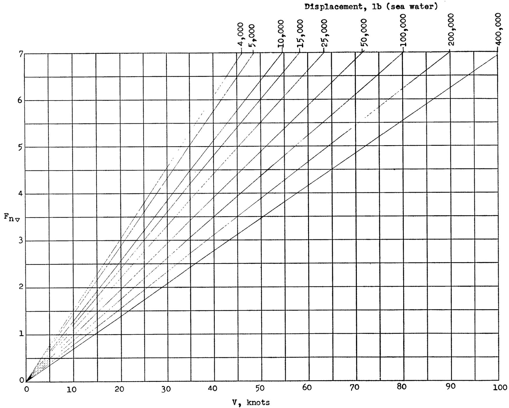
Figure 22. Variation of  $F_{nv}$  with Speed and Displacement
