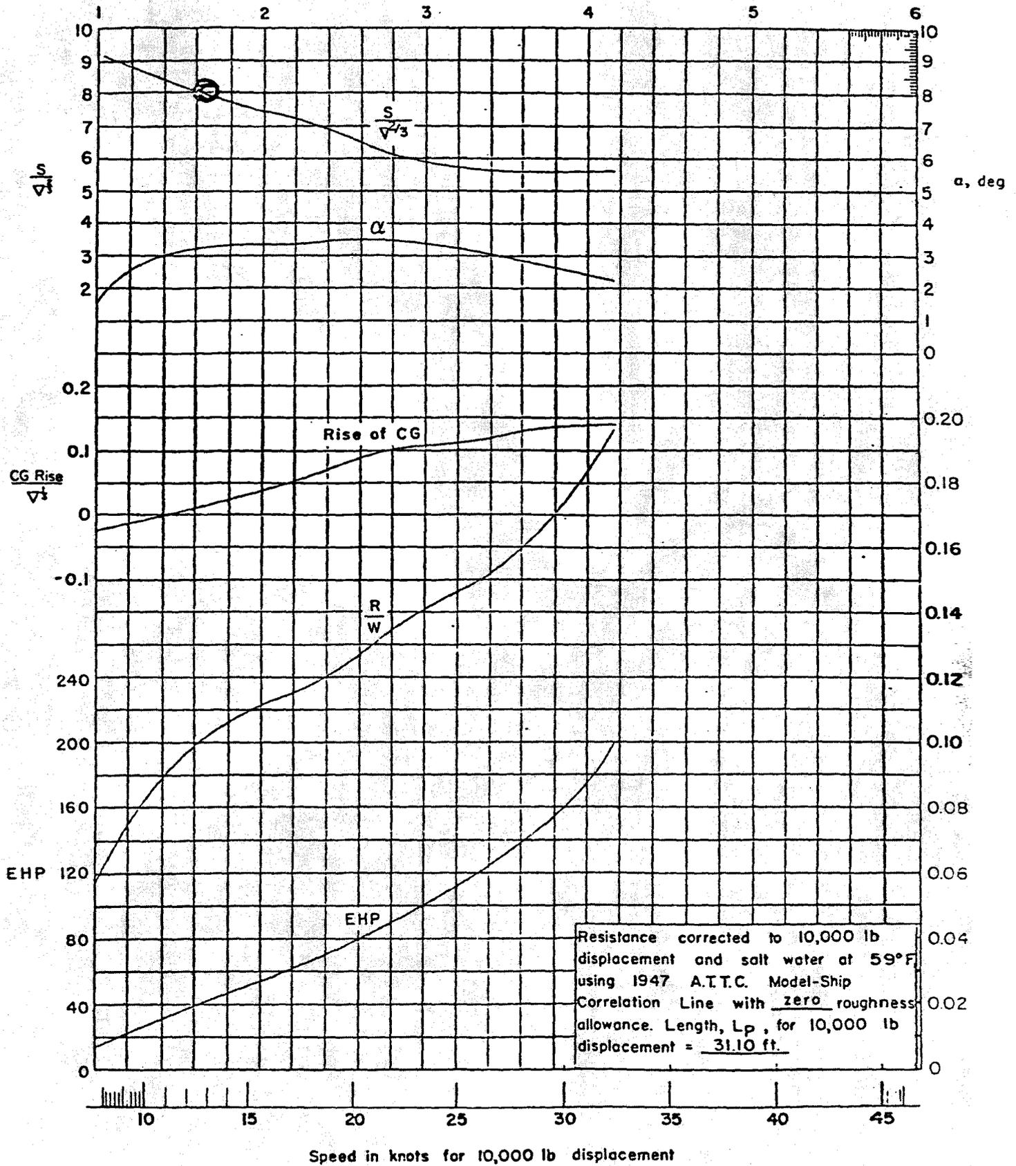
Resistance corrected to 10,000 lb displacement and salt water at 59°F using 1947 A.T.T.C. Model-Ship Correlation Line with zero roughness allowance. Length,  $L_p$ , for 10,000 lb displacement = 31.10 ft.
