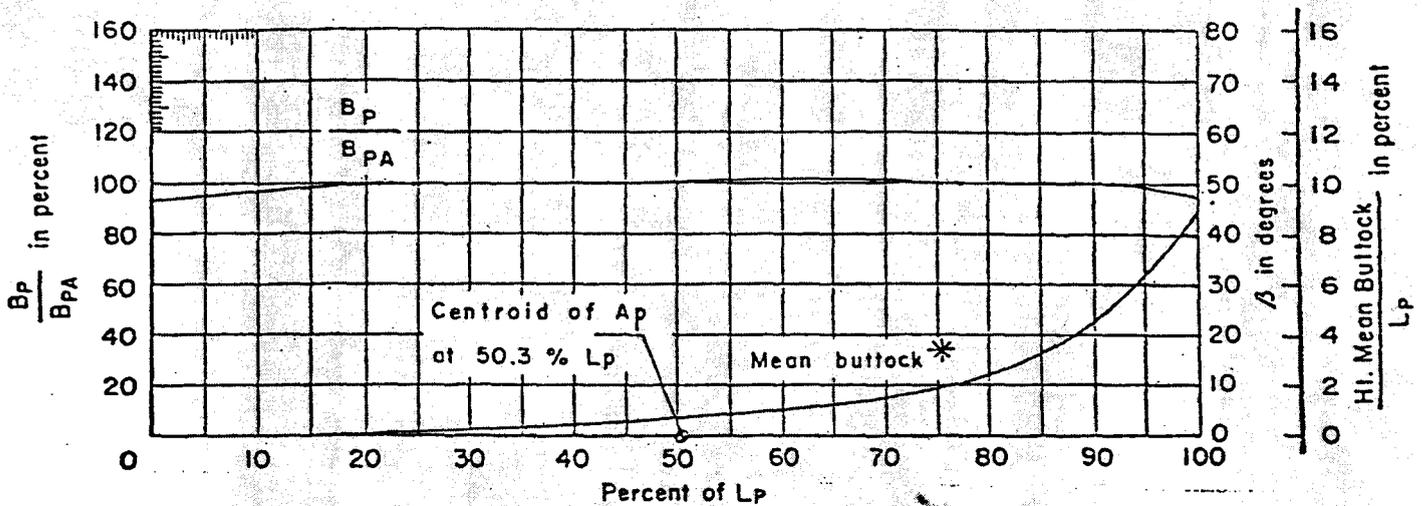
\* Note: The mean buttock as shown is based on the actual body plan instead of a simplified body plan
