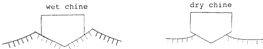
Figure 3.5: Flow conditions around the hull
